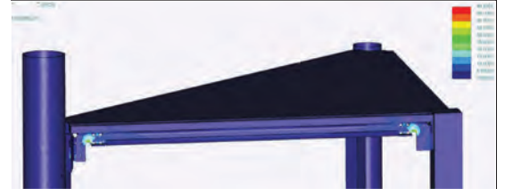
BoldVu® Structural Finite Element Analysis
