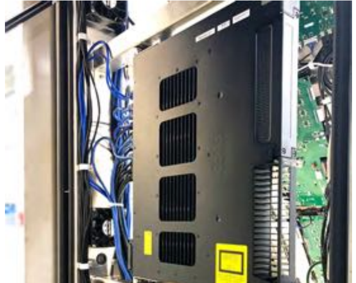
CISCO IE5000 SWITCH INTEGRATED WITHIN THE BOLDVU® SMART POINT ENVIRONMENTALLY SEALED ELECTRONICS CHASSIS.
